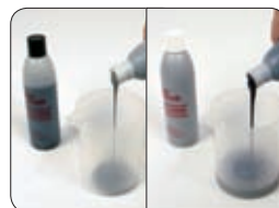
Mix the 2 components in a ratio of 1:1.
