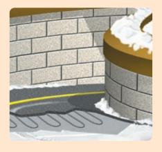
MCA Ramp Self-regulating heating cable for tracing ramps and stairways
