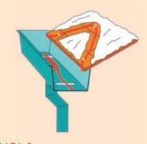
MCA8 Self-regulating cable for tracking roofs, gutters and/or downpipes
