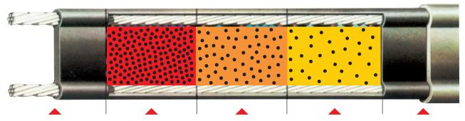
The cable will never become overheated and burn, as it is self-protecting. There is also no need for a thermostat. Almost all the contacts are interrupted by microscopic dilatation of the core at very high temperatures. The electrical resistance becomes very high and energy output is virtually nil.
