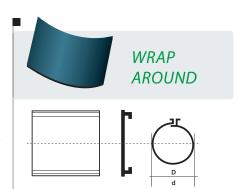
D = 0 minimum before shrinkage  $\mathbf{d} = \emptyset$  maximum after free shrinkage
