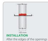
After the edges of the openings have been cleaned, shake the can for at least 30 seconds, then turn upside down and spray the product.
