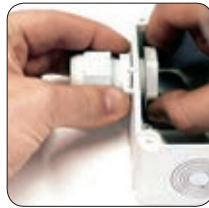
Install the cable glands.
