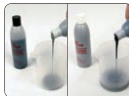
Mix the 2 components in a ratio of 1:1.
